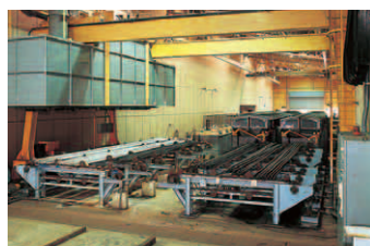
酸洗 Acid Pickling
